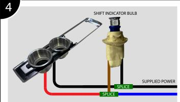
Splice the cupholder wires in with the shift indicator bulb and the wires powering the bulb according to the diagram.
