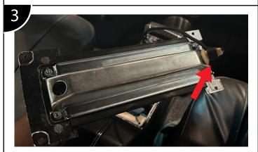
Remove both bulbs from the shift indicator plate. Replace one of the bulbs with the supplied LED bulb. Only one bulb is needed, as the LED bulb is significantly brighter than original.
