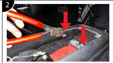
Cut away the two tabs in the center console that interfere with the cupholder kit using side-cutter pliers or a dremel.
