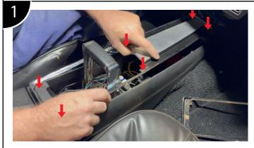
Remove the six screws from the center console plate and remove the plate from the center console.
