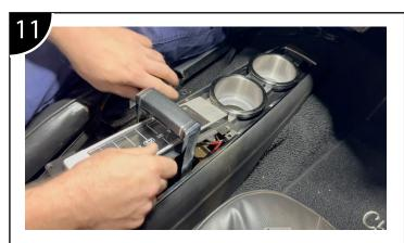
Reassemble the center console with the new assembly. If fitment is too tight, some modification for perfect fitment with OEM center consoles may be needed.
